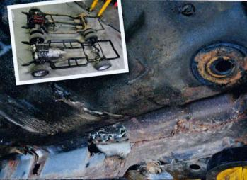
Out with the old, in with the new. MCF ordered this chassis to accommodate a 4L65E four-speed auto and LS3, which bolted straight in. It's easier to fit them now rather slotting them in later. Removing the chassis revealed some serious rust issues, which is very common. In reality this Chevelle was in pretty good condition overall but the corroded areas needed repair before the fit-up could continue
