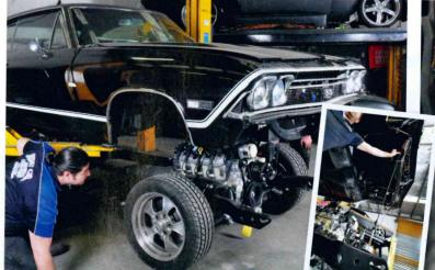
the bolts securing the body to the chassis are undone, lift the body free.
