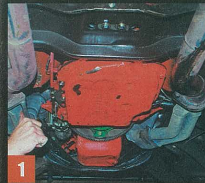
Aftermarket extractors almost always need to be detached before removing the engine.
