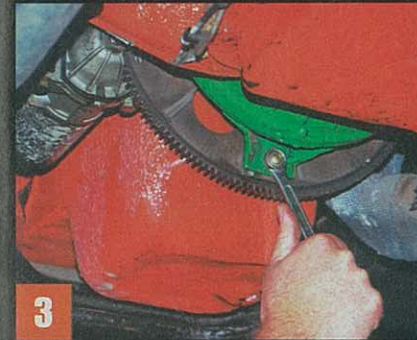
The torque converter must be separated from the flexplate. We'll cover manual transmissions in a couple of issues when we show you how to replace a clutch.
