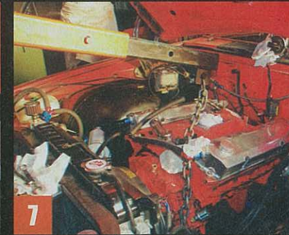
Rags or other padding between chains and other components are essential to protect them.
