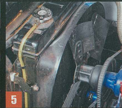
Remove all coolant hoses, fan shrouds, fans and the radiator.
