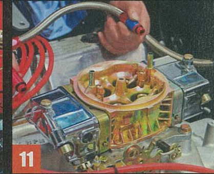
Always use new hoses, clamps and the like when re-fitting an engine and peripherals. Your project deserves it.
