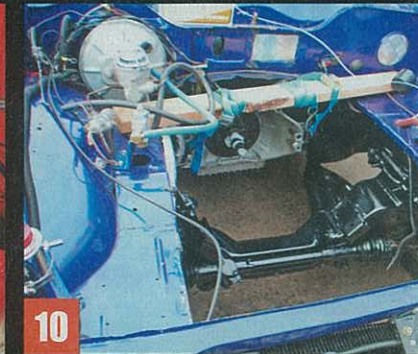
...however, a jack is not a good long-term support for a transmission.
