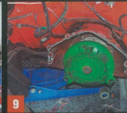
Use a jack to support the transmission during engine removal and installation...
