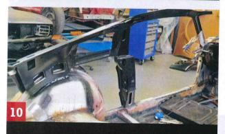
The first test fit of the new side section to the original body. The factory B-pillar support mates with the section of the Taiwanese B-pillar that was cut away in the previous shot. Drill screws and clamps holds everything in place at this stage.
