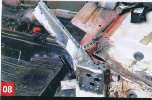
George has unpicked and removed the lower outer section of the B-pillar ready to accept the B-pillar section that's part of the Taiwanese replacement panel.
