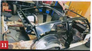
Leo sets roof section cross-braces in place. These are clamped with Visegrips and may have to be reset several times before the transverse dimensions of the new panels are correct. Careful measurement will be required to match the cross-braces to the new sides of the car. The boot divider is also set in place and used to determine the width.
