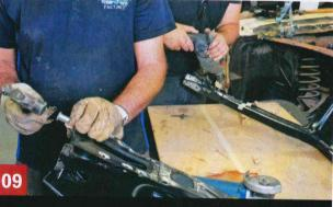
The B-pillar on the aftermarket panel assembly extends right to the sill. Because the old B-pillar support was left sandwiched in the body, this bit has to be removed from the aftermarket panel. This is being unpicked to avoid holes in the panel.
