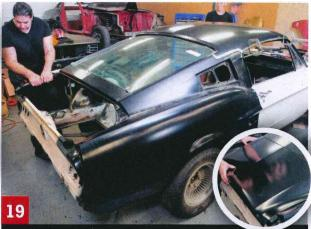
The boot lid was set in place but it was a bit tight at the sides. If it won't fit, bend it. Leo is simply rolling the tops of the guards upwards and outwards simultaneously with a bit of brute force. Fitting can be like this.
