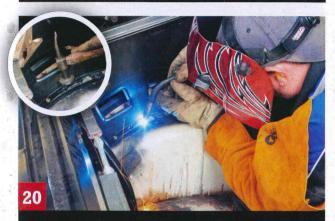
With the job shaping up, more serious welding begins. The inset shows the flanges atop the wheel wells being given a final tap into place before the final puddle welds are made. As we've described in many stories, drill screws are used to hold panels in place temporarily where clamps won't fit.
