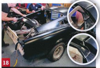
Leo and George make sure the deck lid filler panel is the same distance from the top of the window frame on both sides. The only way the panel would fit was by partially cutting, hammering and bending it. That's what fitting Taiwanese (and original factory) panels is all about.
