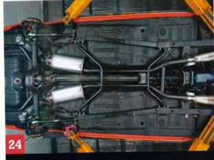
The finished job showing the kits and a superb exhaust system from Trikfab (03) 9792 1333. There's also a tailshaft loop that bolts in above the X-brace. You can call The Muscle Car Factory on (03) 9580 3548 or visit musclecarfactory.com.au
