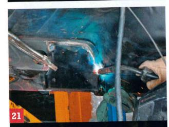
On this side just one clamp was used, however, the RHS under the rag just beneath the weld leads down to a trolley jack. It's jacking the reinforcing rail up against the floorpan/body rails using the weight of the car to hold the reinforcing rail in place.
