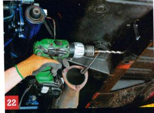
With the welding completed, holes are drilled in the body rail to fix the X-brace in place. Note that the body rails may have undergone considerable rubber mallet persuasion to adjust their width so that the X-brace fits neatly at this stage.
