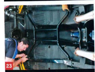
The body rails aren't hit directly but rather through blocks of wood against them to protect them from damage. Trial fits of the X-brace are made prior to welding at all stages so that this last operation goes smoothly.
