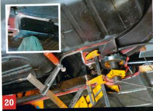
Here's one solution for holding the rear-end of the reinforcing rails in place. Note that before the rear ends are welded in place, the front ends have just one bead applied across the front edge. It holds it in place but also acts as a very stiff pivot.
