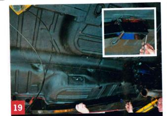
Now the connecting rails and X-brace have to be fitted. As with the rear kit, the areas in which these components have to be welded is cleaned up. So, set the rails in place and mark areas that must be taken back to metal.
